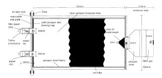
**Fig. 1.** Bioassay apparatus: b and c are the points of entry for the air flow into the bioassay tube, a is the exit point for the air flow and d is where the sandflies are introduced into the apparatus. For clarity the apparatus is not drawn to scale (see text for details).
