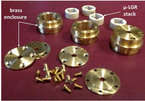
Fig. 6. Some of the built prototypes based on the \mu -LGR optimized solution.
