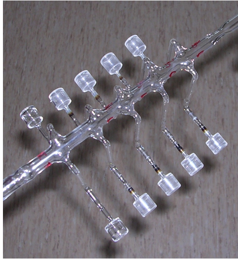
FIGURE 5.1: Parylene ramp before being filled with rubidium.
