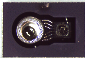
Figure 3.15: Example of a cell with excess Rb due to a too high laser intensity and too long activation time (6W for 20s)
