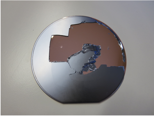
Figure 3.9: Bonding test of silicon on sapphire: silicon substrate broken due to the too high CTE difference
