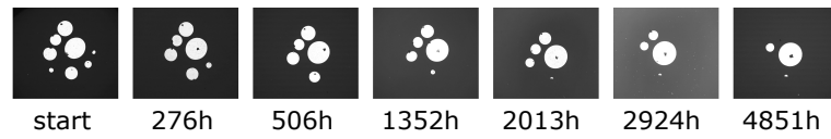
Figure 5.3: Example of the droplets evolution over time for a cell heated at 196°C. Small black dots can be observed on each drop. These particles of unknown composition are likely the nucleation sites of the droplets. - Microscope image: courtesy of Jean Gobet, CSEM - Copyright © 2017 Optical Society of America. Reprint by permission of Optical Society of America.
