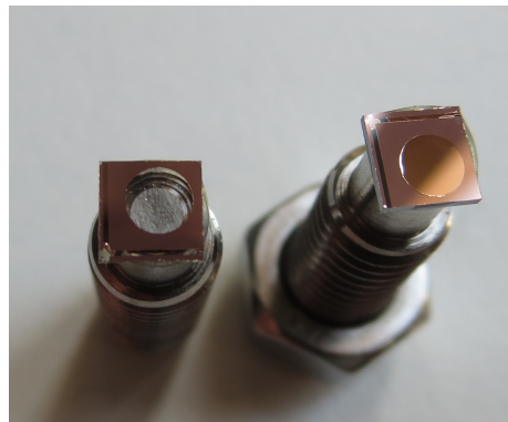
Figure 3.6: Example of a bonding sample of run 2 after the pull test: The Cu layer did not adhere to the glass substrate
