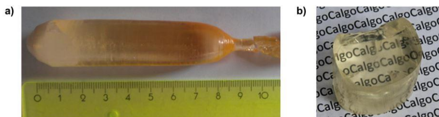
Figure 20. Large-size Yb:CALGO crystals grown by the Czochralski method. a) Crystal boule and b) bulk Yb:CALGO crystal. Picture courtesy of C. Kränkel.
