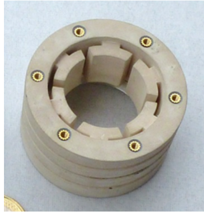
Figure 4.1 – Photography of the AdM microwave cavity manufactured using SLA technology (metal-coated polymer). Figure adapted from [109].
